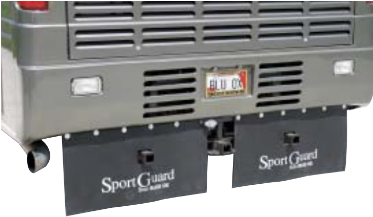
ADDING LARGE RUBBER FLAPS AT THE REAR OF A MOTORHOME WILL MINIMIZE TOWED-VEHICLE DAMAGE FROM DEBRIS, DIRT AND GRIME KICKED UP BY COACH TIRES.
