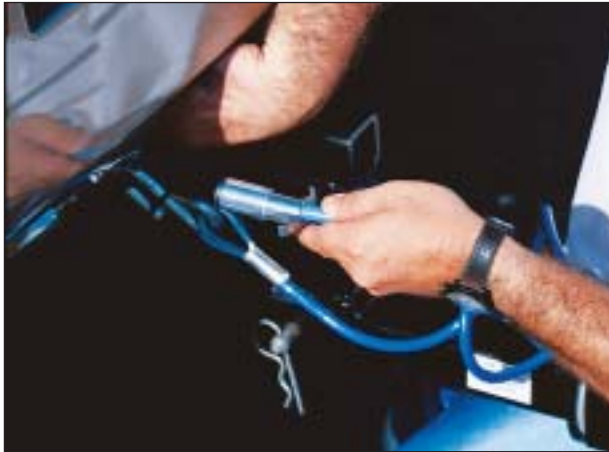
PLUG RECEPTACLES ADDED TO DINGHY AND MOTORHOME ALLOW EASY HOOKUP OF ELECTRICAL CONNECTOR FOR TAILLIGHTS, TURN FUNCTIONS AND SUPPLEMENTAL BRAKING SYSTEM.
