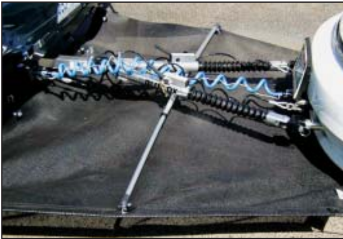
AN RV UNDERSKIRT WILL KEEP TOWING APPARATUS CLEAN — AND IT ALSO HELPS PROTECT THE FRONT OF THE TOWED VEHICLE FROM ROAD DEBRIS.
