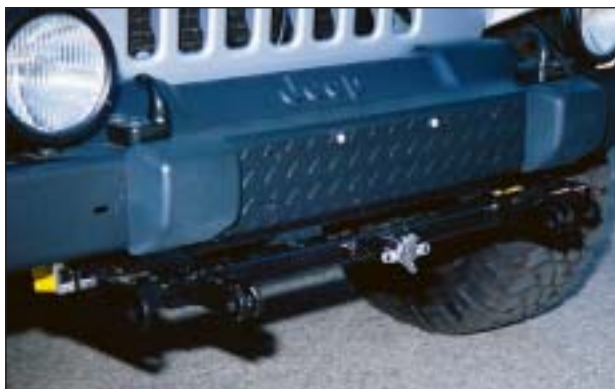
ONCE THE PROPER BASEPLATE IS INSTALLED, THIS CLEAN-LOOKING SETUP IS ALL THAT REMAINS WHEN THE TOWED VEHICLE ISN'T HOOKED UP; COOLING DOESN'T SUFFER.
