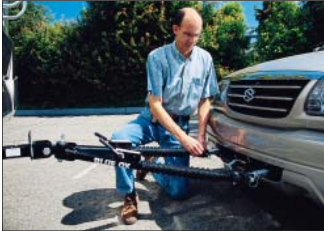
THE TOW BAR ATTACHES TO DINGHY QUICKLY AND EASILY WITH A PAIR OF HITCH PINS; TELESCOPING BARS FURTHER EASE THE HOOKUP.
